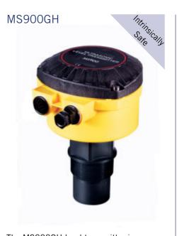
The MS900GH level transmitter is intrinsically safe certified for use in hazardous areas. Power must be supplied through a suitable I.S. barrier. Hart digital communications are also provided.
