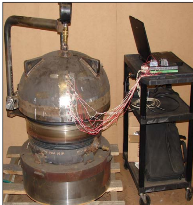
24" CL900V Closure under 3350 psi Hydrostatic Test
